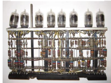
FIGURE 8-23: VACUUM TUBES USED TO STORE AND PROCESS DATA
