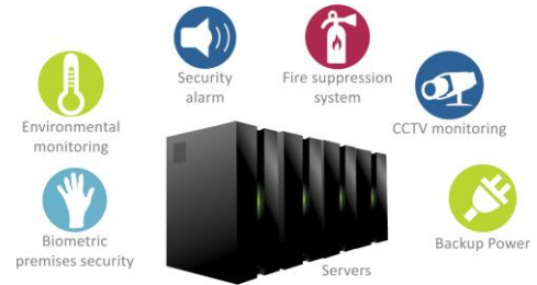
FIGURE 9-49: DATA CENTER COMPONENTS
