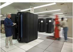
FIGURE 1-20 This IBM z9 mainframe computer weighs 2,807 pounds and is about 6.5 feet tall.
