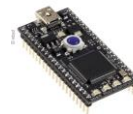
FIGURE 1-22 A microcontroller is a self-contained chip that can be embedded in an appliance, vehicle, or other device.
