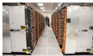
FIGURE 1-21 In 2010, IBM Blue Gene/Q became the fastest supercomputer in the world. With a speed of 16.32 petaflops, the number of calculations the computer can perform in one hour would require 300 years if done one way on Earth using a handheld calculator.
