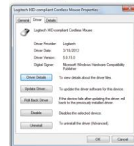
FIGURE 3-18 The Windows Device Manager offers access to device drivers. You can check if they are working and change settings. You can also check the device driver's version number and compare it with the most recent version posted online.
