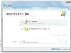
FIGURE 4-58 Disk imaging software, such as Acronis True Image, creates a bit-by-bit copy of all the data on your computer's hard disk that can be used to restore all operating system, program, and data files.
