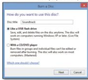
FIGURE 4-50 CDs and DVDs can be created using mastering or stamping techniques. Mastering creates discs that can be used more reliably on a wide variety of computers and standalone players. Stamping is more flexible for discs that you plan to use only on your own computer.
