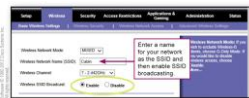
FIGURE 5-30 Create an SSID for your network so that it can be differentiated from other nearby networks.
