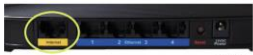
FIGURE 5-34 Look for a port labeled "WAN" or "Internet" on your router. If one does not exist, then use any of the other Ethernet ports.
