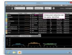
FIGURE 5-51 Software tools such as WiScrub help locate and identify secured and unsecured networks. Once logged on to an unsecured wireless network, hackers are free to do anything from stealing the network owner's credit card or bank information to attacking computers in other networks.
