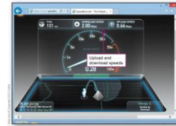
FIGURE 6-13 Speed tests measure the average number of bits that are transmitted per second, whereas utilities such as Ping and Traceroute measure the time required for a packet to make a round trip from your computer and back. Click to learn how to use Speedtest.net to compare the speed of your Internet connection with your ISP's advertised speed.
