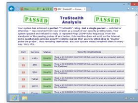
FIGURE 6-40 Your computer's ports are most secure if they don't even appear to exist when probed using a port scanner. Use your interactive block to see how ShieldsUP! checks your computer's ports and learn what the results mean.
