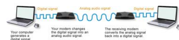
FIGURE 6-15 When you transmit data, your voiceband modem modulates the signal that carries your data. A modem at the other end of the transmission demodulates the signal.
