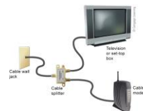
FIGURE 6-21 If your home has only one CATV cable outlet, you might need to use a splitter to link it to your cable modem and television. If you have multiple cable outlets, you can connect your cable modem directly to any one of them.
