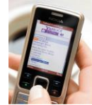
FIGURE 6-30 The advantages of WAP-enabled devices include their portability and low price. The disadvantage is their small, low-resolution screens. Although various schemes for scrolling over a full-sized Web page have been tried, most WAP users click to Web sites specially designed for small screens.
