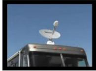
FIGURE 6-29 A vehicle-mounted satellite dish can be deployed from a control panel inside the vehicle. As with fixed satellite service, however, latency becomes a factor for real-time applications such as videoconferencing, streaming music, and online gaming.
