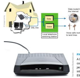
FIGURE 6-16 Voice and data signals travel over DSL to a special device at the local telephone switching station, where they are divided and routed to an ISP or to the regular telephone network.
