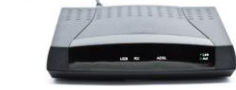
FIGURE 6-18 A DSL modem connects your computer to a telephone wall jack. You can plug the modem into your computer's USB or Ethernet port.
