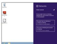
FIGURE 6-27 When connecting to a new Wi-Fi network, Windows gives you an opportunity to turn the sharing off. If the network is public and secure you can have the sharing on. But if the network is public or unsecured, then select the option to enable sharing.
