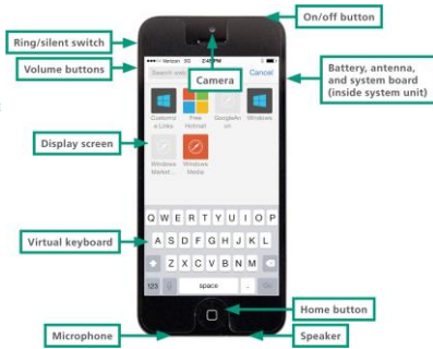
FIGURE 2-10: A TYPICAL SLATE DEVICE
