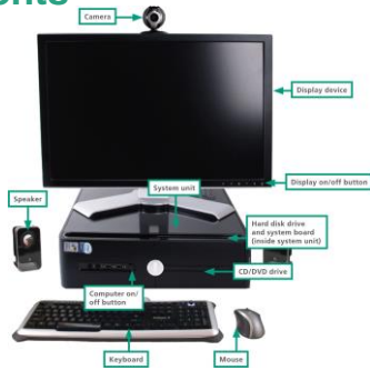
FIGURE 2-8: A TYPICAL COMPONENT SYSTEM
