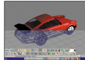
FIGURE 8-38 3-D graphics software provides tools for drawing a wireframe and then specifying colors and textures for rendering. Flash's wireframe being rendered and animated in your interactive eBook.
