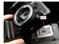
FIGURE 8-12 A digital camera's CCD converts the image captured by the camera lens into a grid of colored pixels, which are stored as bits. Watch the video for this figure in your interactive eBook for an overview of digital camera features, the formats, and the process of transferring photos from a camera to your computer.
