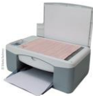
FIGURE 8-13 To scan an image, turn on the scanner and start your scanner software. Place the image face down on the scanner glass and then use the scanner software to initiate the scan. The scanned image is saved in RAM and can then be saved on your computer's hard disk. Learn the difference between scanning an image and scanning a document into an editable word processing file.
