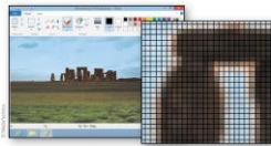
FIGURE 8-11 A bitmap graphic is divided into a grid of individually colored pixels. The color number for each pixel is stored in binary format. Watch the video for this figure in your interactive eBook for an overview of digital camera features, the formats, and the process of transferring photos from a camera to your computer.
