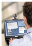
FIGURE 8-43 A Web camera can be built into a computer display device or can be attached as shown. It is designed mainly for "talking head" applications, such as online video chats and video-conferences.
