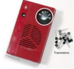
FIGURE 9-8 Transistors first sparked a revolution in the entertainment industry by providing a small, power-efficient technology for portable radios. Later, transistors were incorporated in computers to replace large, hot, power-hungry vacuum tubes.
