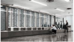
FIGURE 9-8 Constructed of relay switches, rotating shafts, and clutches, the Harvard Mark I resembled the a "roomful of ladies knitting." The device was 51 feet long and 6 feet tall and weighed about 5 tons.
