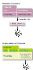
FIGURE 11-18 A relational database serves as the basis for an object-relational database. (top), but an object-relational database can store the song data and the routine to play it.
