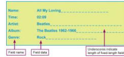
FIGURE 11-7 When setting up a database, the length of text fields should be adequate to store the longest names or files. The Time field can be short because the longest tracks are 60 minutes or less, which can be expressed in the format MM:SS, where MM is minutes and SS is seconds.
