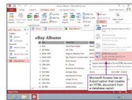
FIGURE 11-24 Many entry-level DBMSs include an easy way to turn a report into an HTML document that you can post as a Web page. Learn how to generate an HTML report from a Microsoft Access database.
