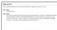
FIGURE 12-55 This verbose error message provides attackers with information about restricted access, folder names and locations, as well as account names (Manager, Member, and Owner) that can gain access to these folders.
