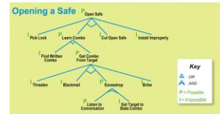
FIGURE 12-58 Attack trees are used by security analysts in many fields. This diagram illustrates an attack tree that might be devised by a bank security officer examining the vulnerability of the bank vault.
